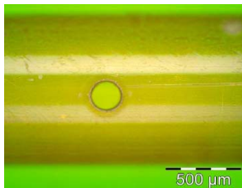
Fig 2. A 210 µm hole machined in 51 µm wall polyimide tubing.
